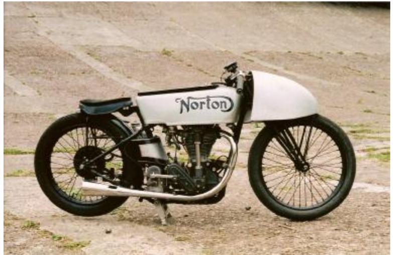
One is a replica of the bike ridden by Jimmie Guthrie at Monthéry in October 1935, when he broke the classic hour record at a speed of 114.09 mph. It was fitted with a seven gallon fuel tank and ran on alcohol.
