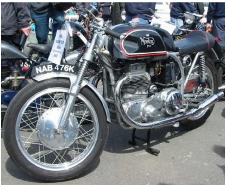
This Norton Four, using an Ariel square 4 motor squeezed into the Norton frame was on sale for £6995.
